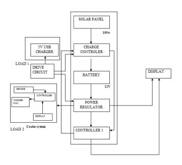
SOLAR:Here we use photovoltaic solar panel. Photovoltaic solar panels absorb sunlight as a source of energy to generate electricity. A photovoltaic (PV) module is a packaged, connected assembly of typically 6x10 photovoltaic solar cells. Photovoltaic modules constitute the photovoltaic array of a photovoltaic system that generates and
