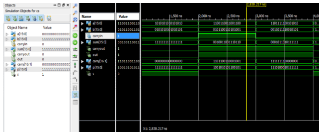
Figure 6: Output of carry skip adder
