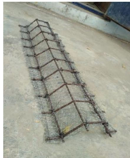
Fig. 3. Skeletal steel with wire mesh
