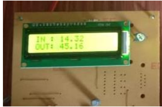
Fig. 8 Input and Output voltage
