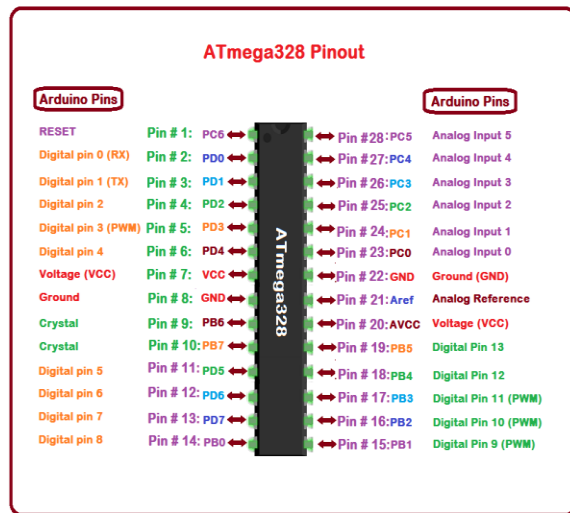
Fig. 5 Atmega328-Pinout
