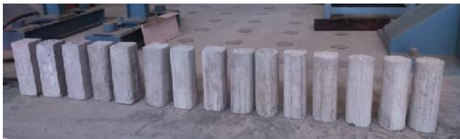
Fig7.1 Unconfined Concrete Column Specimen With Varying Corner Radius
