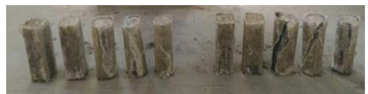
Fig 7.4 failure crack pattern of single and double layer FRP confined concrete column with varying corner radius (Sharp Edges, 15mm, 25mm, 35mm And 62.5mm)
